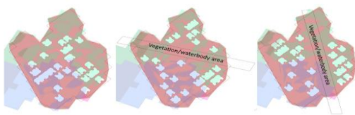
Figure 10: Illustration of vegetation areas exclusion As shown in Figure 10, the script will automatically avoid creating buildings in areas that are covered with vegetation or waterbody.
